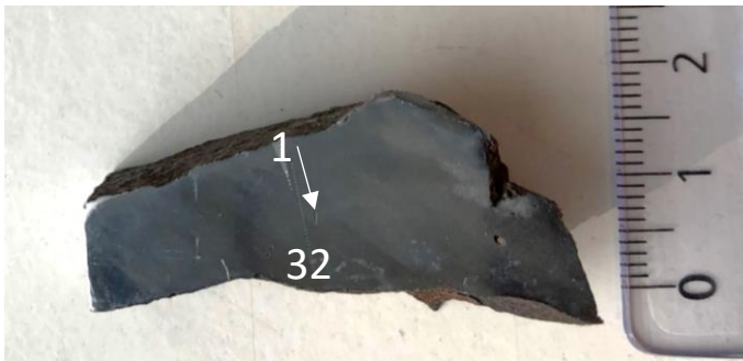
Figure 26 Indication of the hardness measurements across the interface of sample 2.
