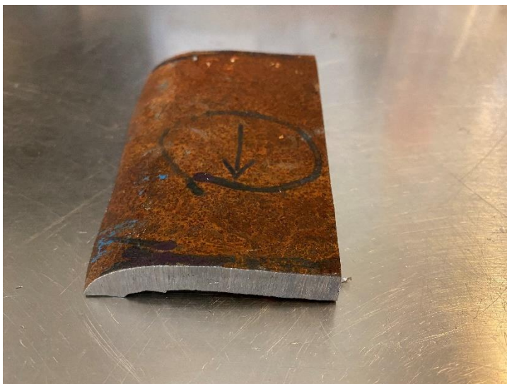
Figure 5 The sample from the unaffected region was taken from the cross section that the arrow points to.
